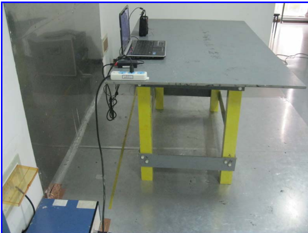
Conducted Emissions Test Setup - Side View
