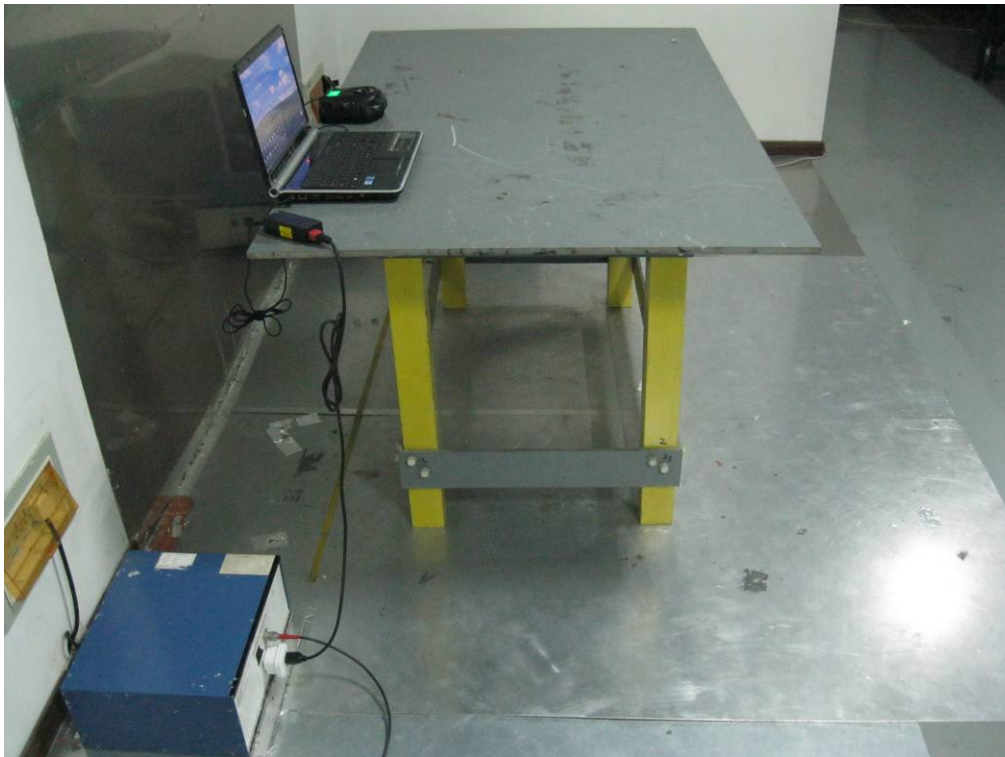
Conducted Emissions Setup Side View
