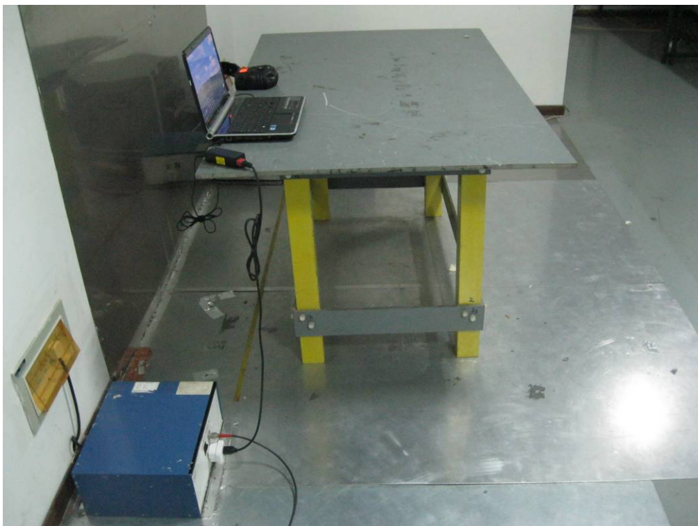
Conducted Emissions Setup Side View
