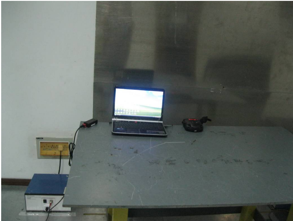
Conducted Emissions Setup Front View
