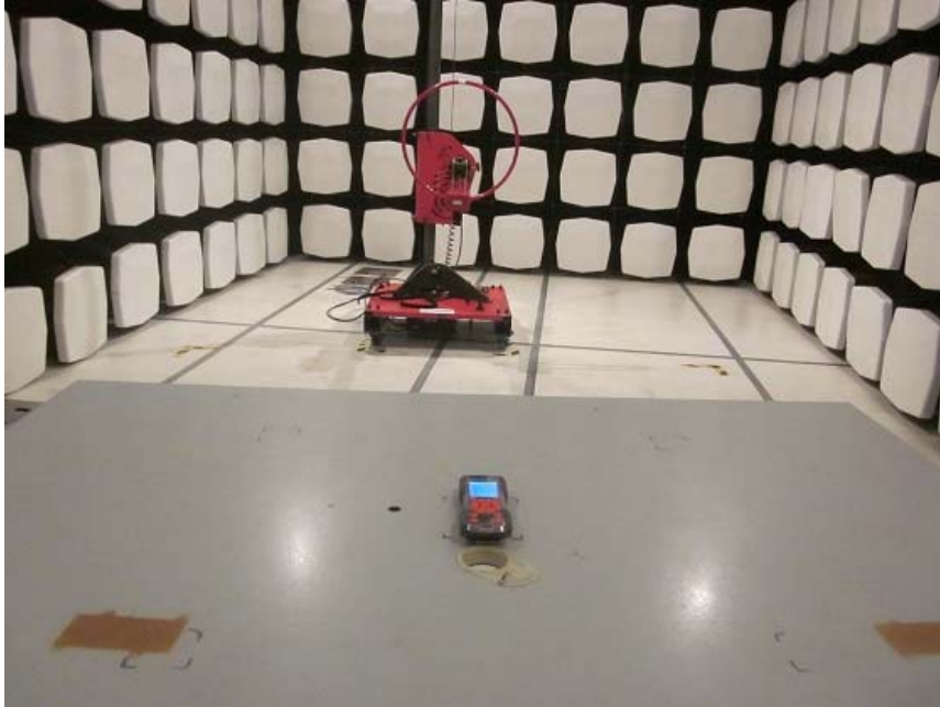
Measurement of Radiated Emission Test Set Up
