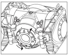
Next, pull out the battery chamber, confirm that the positive (+) and negative (-) terminals are oriented correctly and insert ten (10) AA batteries.
