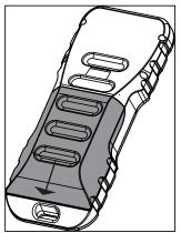
Next, confirm that the positive (+) and negative (-) terminals are oriented correctly and insert the batteries.
