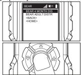
While playing any sound from any location (preloaded, downloaded or sd card) press the FAV1 or FAV2 buttons for 3 seconds to set that sound for the selected FAV button.
