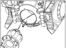
**3**To close put battery chamber back inside cavity while aligning the arrows and rotate to the right till you can't turn it any further.
