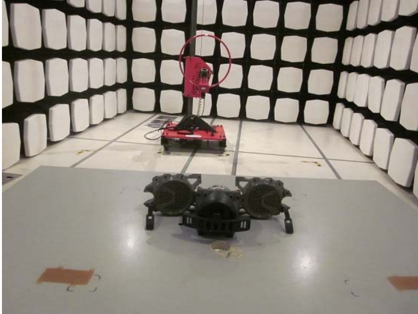
Measurement of Radiated Emission Test Set Up
