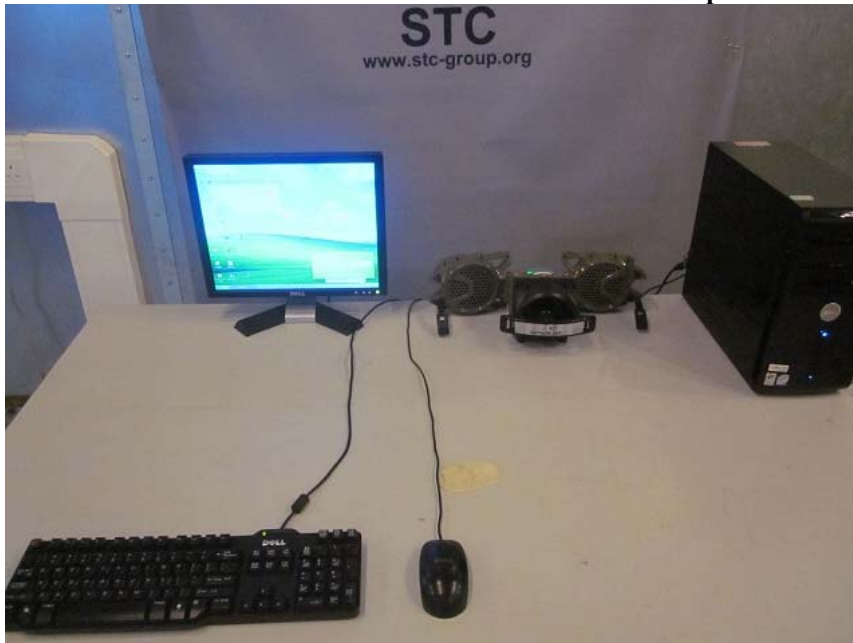
Measurement of Conducted Emission Test Set Up
