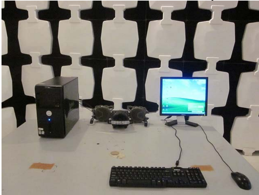
Measurement of Radiated Emission Test Set Up
