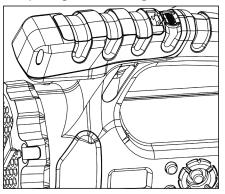
To attach the remote hold with buttons facing down and slide in until it clicks.
