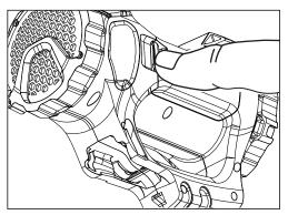
Next, pull out the battery chamber, confirm that the positive (+) and negative (-) terminals are oriented correctly as described on the label at the entrance and insert the AA batteries.
