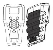
To close, place the cover over and press down. Press the door snap after battery door installment to ensure door snap engagement.
