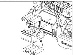
To close put battery chamber back inside cavity, put the cover over and press in. Press the door snap after battery door installment to ensure door snap engagement.
