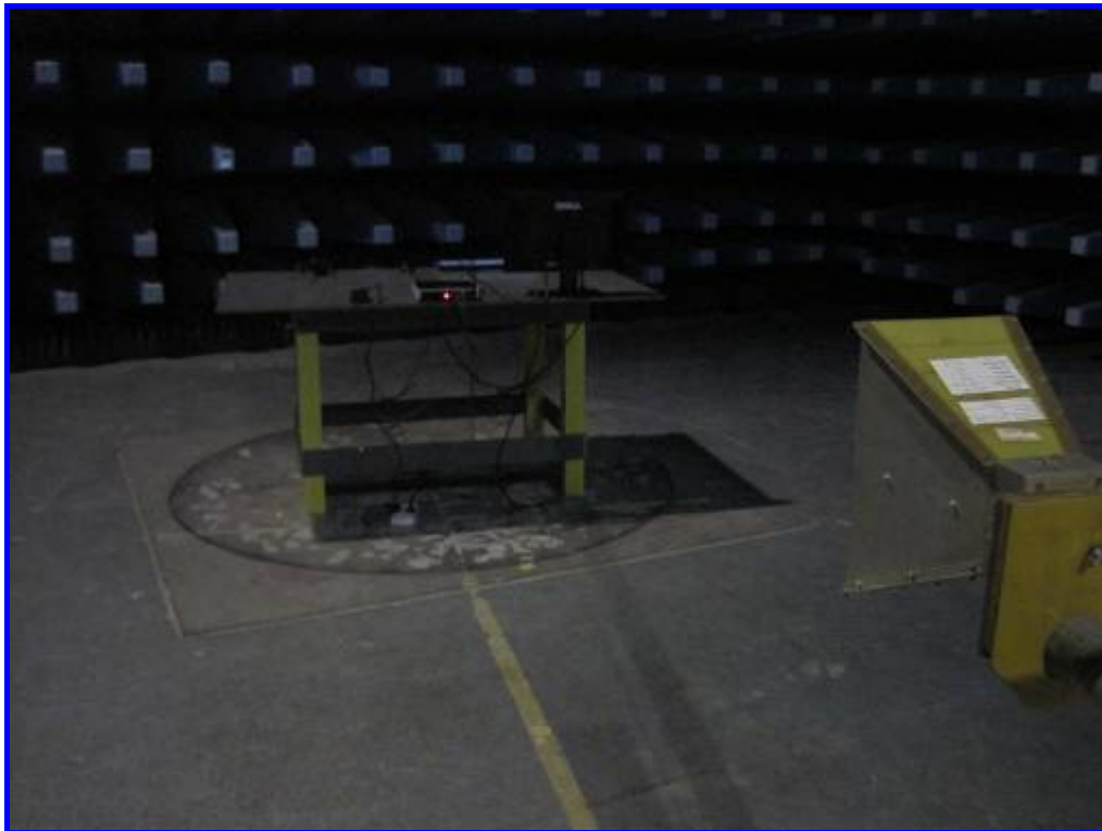
Rear View of Radiated Emission Test Setup above 1GHz
