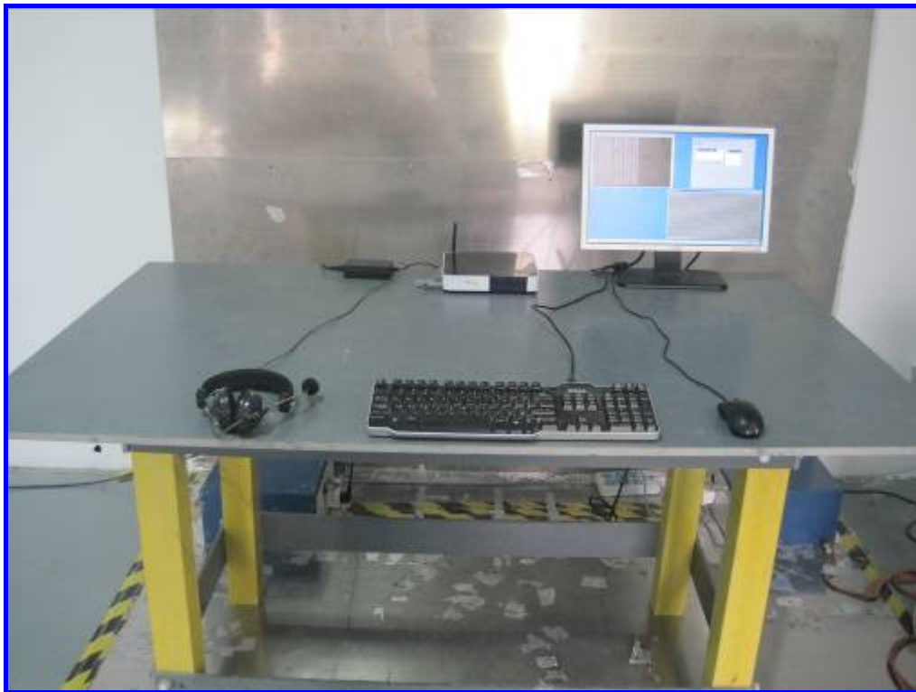
Front View of Conducted Emission Test Setup
