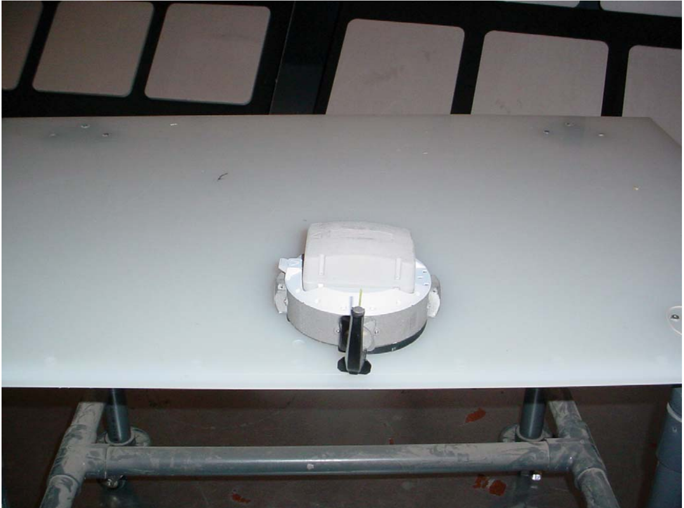
Radiated Emissions @ 3 m Test Configuration for Co-location Transmitters Radiated Emissions, Closed Enclosure
