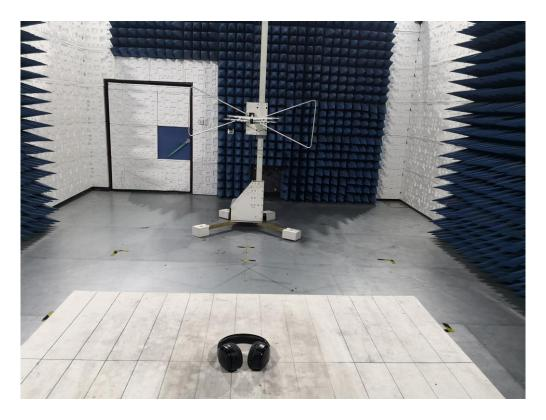
RADIATED EMISSION TEST SETUP ABOVE 1GHZ
