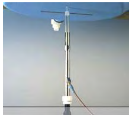
Photograph of the dipole Antenna
