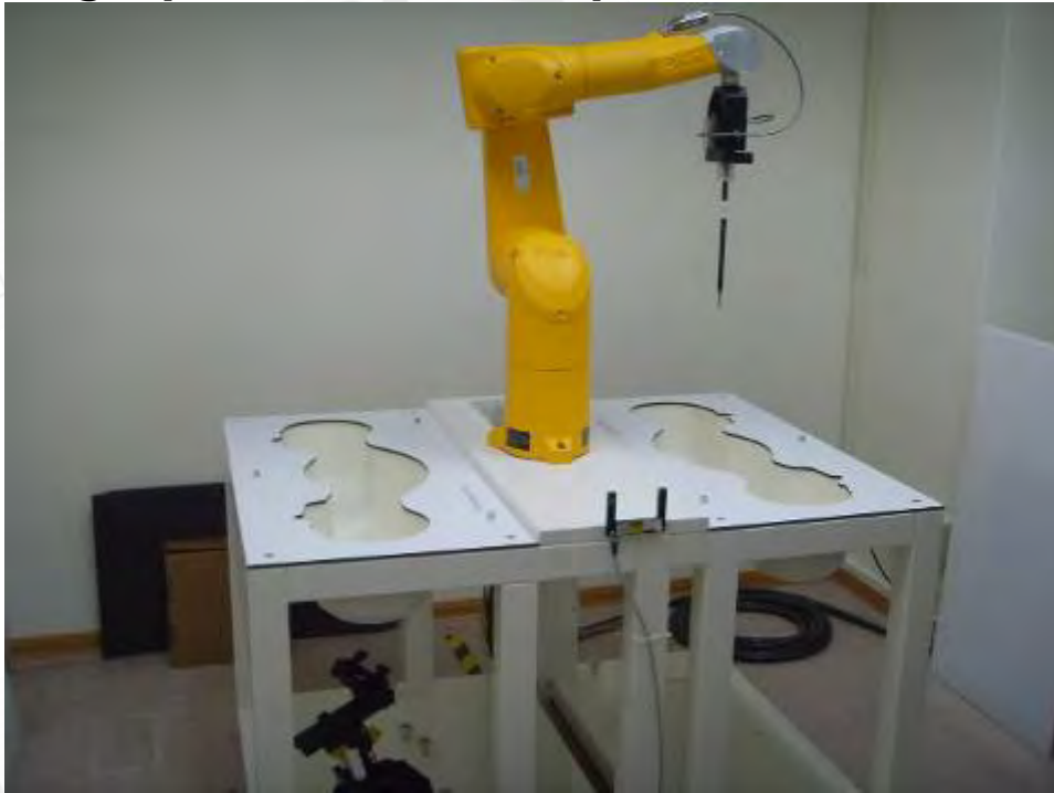
Fig.1 Photograph of the SAR measurement System
