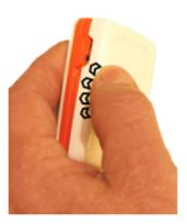
To close Spider SAS clip the right side of the back part into the orange plastic part then apply a light pressure (black arrows) on the left part with your thumb until the back cover is locked (with a click) onto the orange plastic part. Then lock the back side of the Spider SAS (using a screwdriver or a coin).
