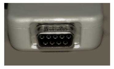
Connect the finger sensor (SpO<sub>2</sub>) cable to the connector located at the bottom of  $\phi$  Hub by pushing it at the maximum. The metal part of the connector is no longer visible and the cable is firmly maintained.
