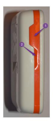
The figure on the left shows how to open Spider SAS in order to access the battery,  $\mu$ SD card, on/off button, connectors for ECG cable and Physio Hub. The patient should be instructed not to remove the cover under any circumstances.
