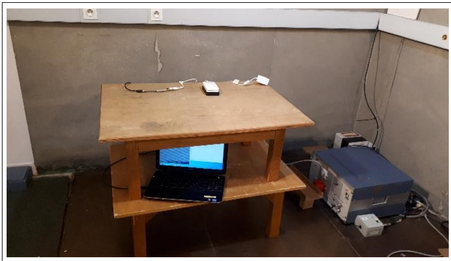
Photograph for AC Power Line Conducted Emissions (Front view)
