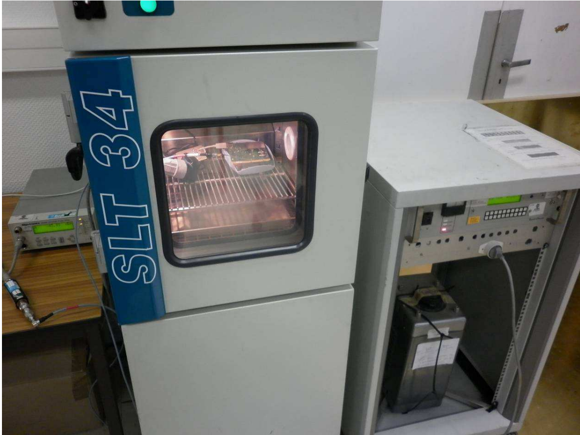
Radio temperature test setup photographs
