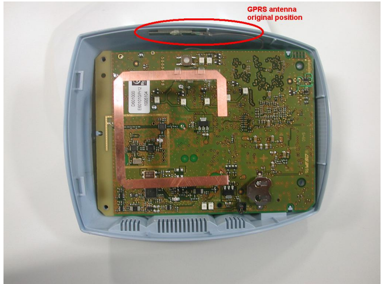
Figure 1.3: The GPRS antenna is originally placed on the On-Demand button HM side.
