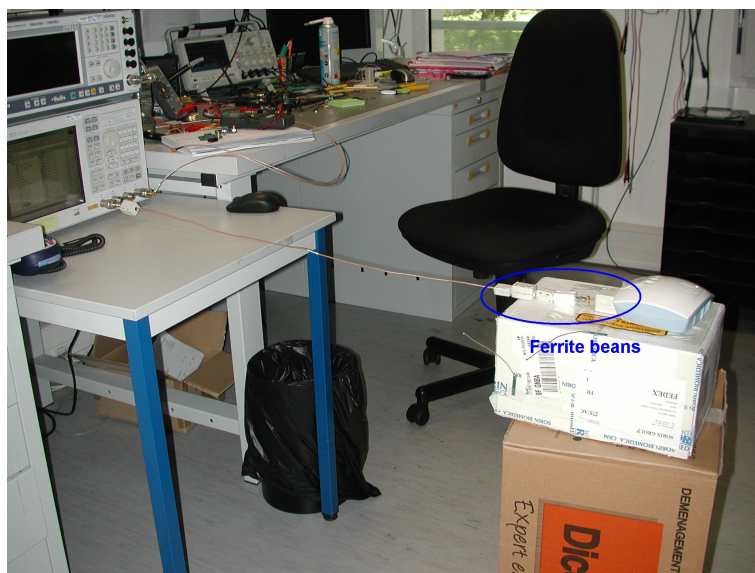
Figure 1.15: Ferrite beans on cable reduces measurement disturbances
