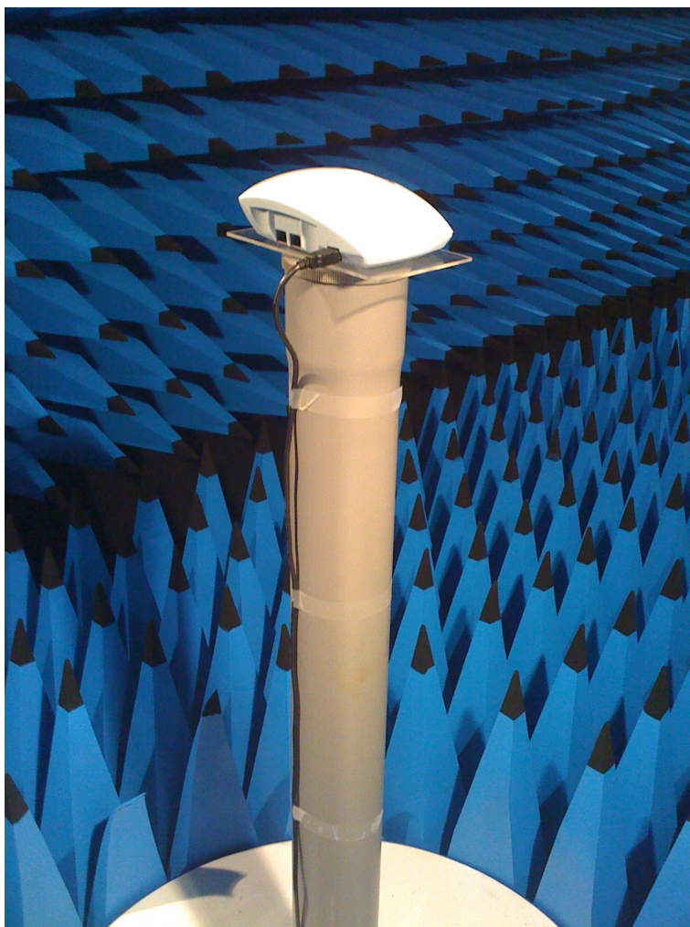
Figure 1.8: The USB cable position is fixed along the support for the radiation pattern measurement.
