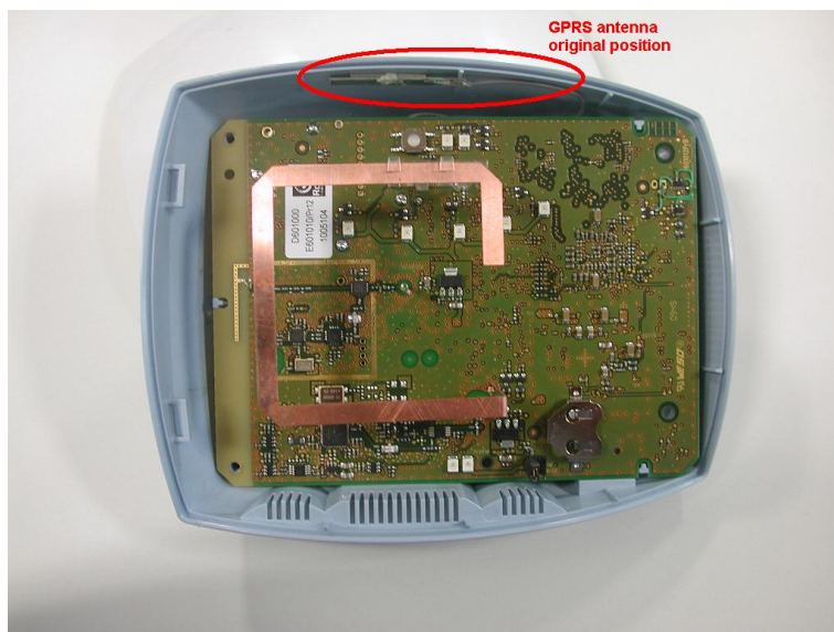
Figure 1.1: The GPRS antenna is originally placed on the On-Demand button HM side.
