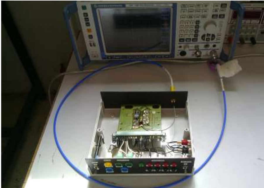
Photograph for RF conducted output power
