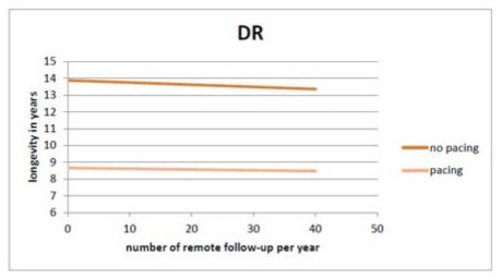
1. An excessive number of remote follow-ups can have a non-negligible impact on device longevity.
