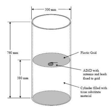
For the testing, the equipment under test (EUT) was suspended in a Plexiglas torso simulator as specified above. The simulator used was constructed in accordance with FCC 95.627(g)(3)(i), EN 301 839-1 (A.113) and EN 301 489-27 annex B.
