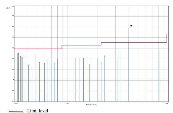
Remark: During the Scan, no unwanted emission has been detected in the frequency range 1 GHz to 25 GHz.
