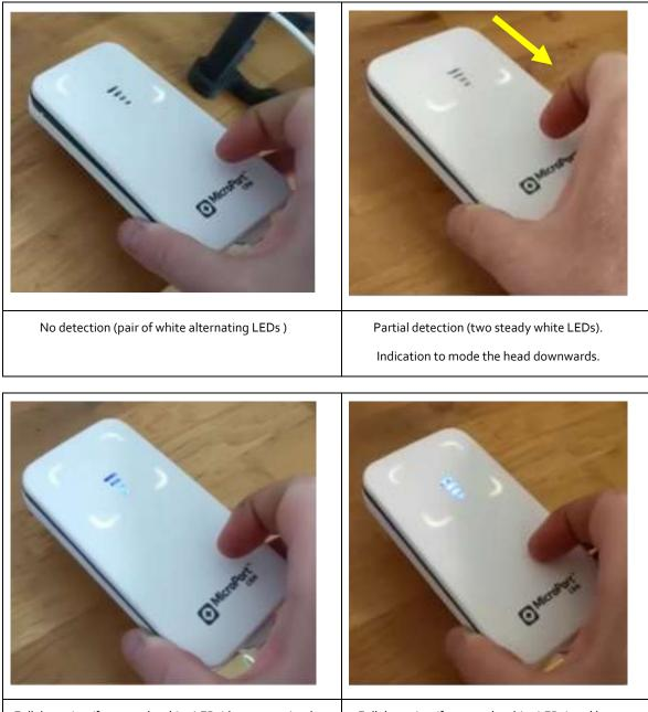
Full detection (four steady white LEDs) but not optimal position (only two blue LEDs)
