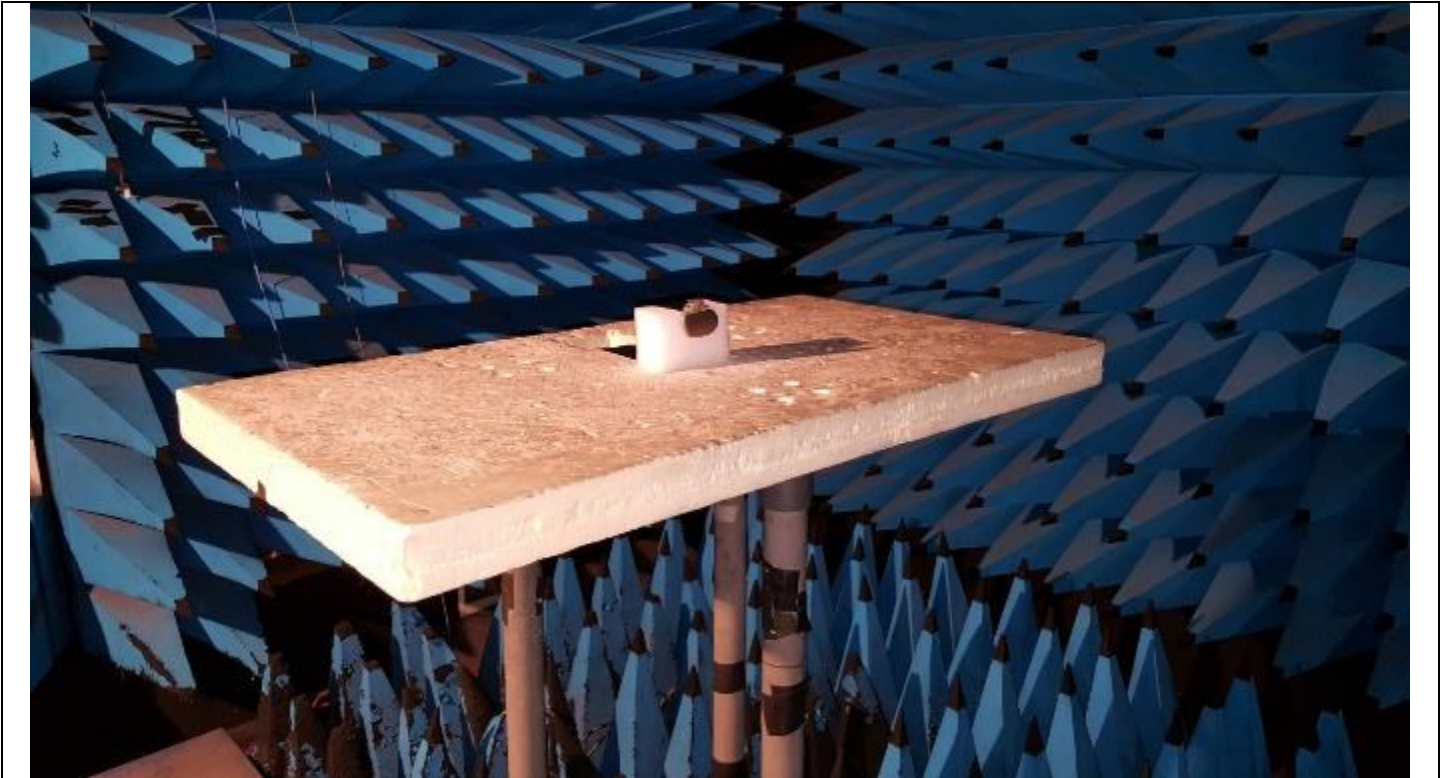
Photograph for Unwanted Emission in restricted frequency bands
