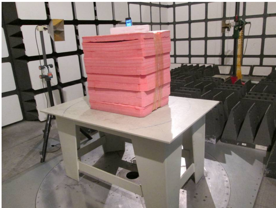
Radiated Emissions Test View (Above 1 GHz)
