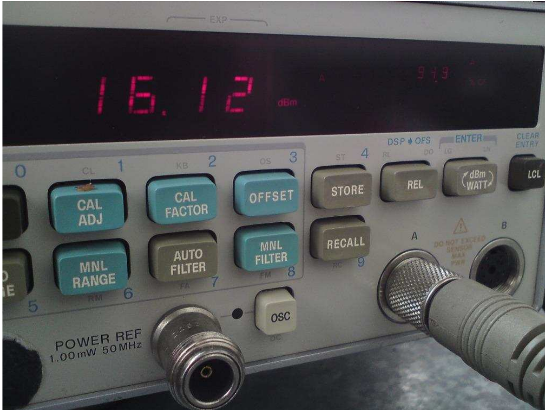
Figure 4: Power meter for RF Peak Power, Low Frequency at TX output (16.12 dBm without cable).
