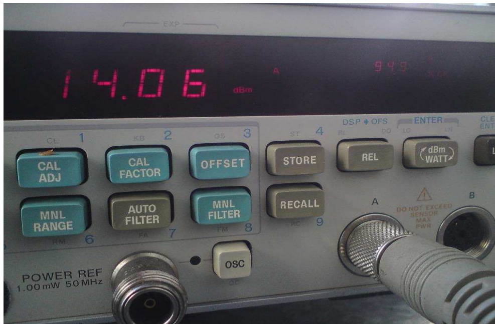
Figure 9: Power Meter Reading for RF Peak Power, High frequency (14.06 dBm using cable).
