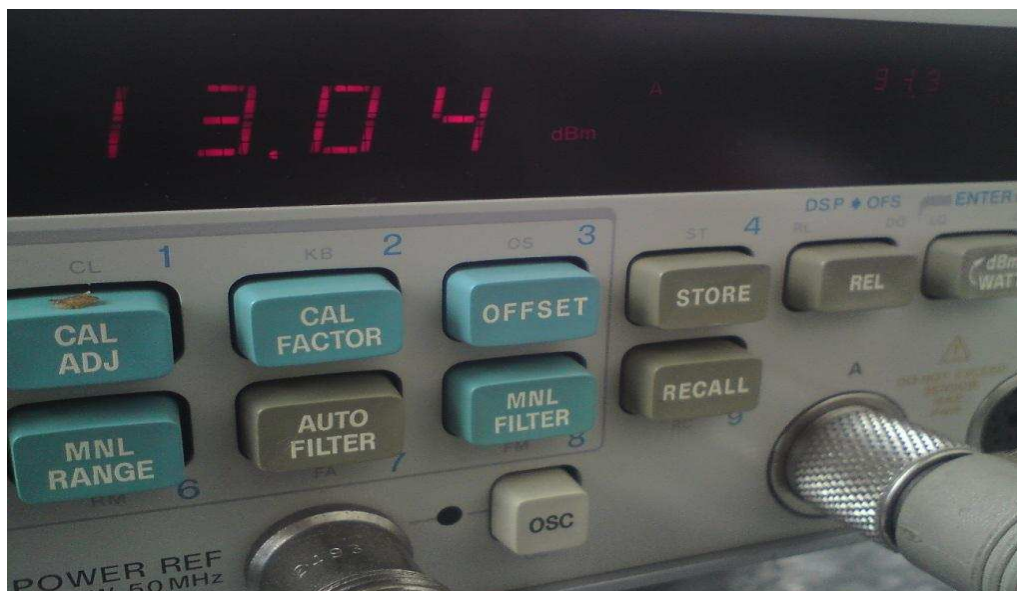
Figure 3 : Power Meter Reading for RF Peak Power, Low Frequency (13.04 dBm using cable)
