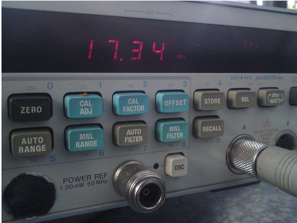
Figure 10: Power Meter Reading for RF Peak Power, High Frequency at TX output (17.34 dBm without cable).
