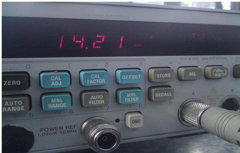
Figure 6: Power Meter Reading for RF Peak Power, Centre Frequency (14.21 dBm using cable)
