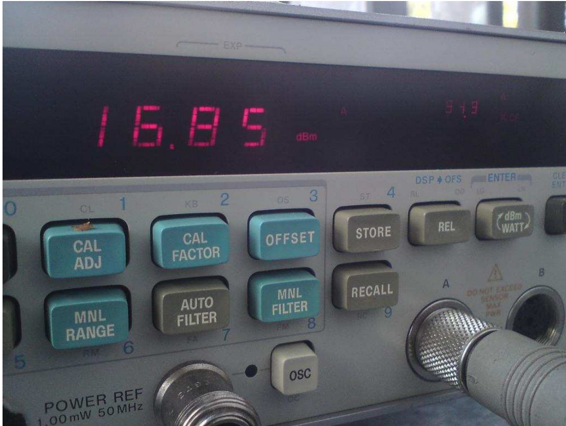
Figure 7: Power Meter Reading for RF Peak Power at TRX output without cable, Centre Frequency (16.85 dBm)
