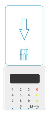
Figure 3 Smart card with the gold contacts upward
