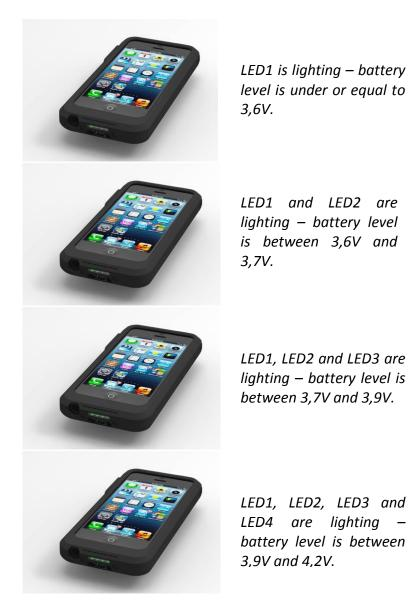
While the device is charged, depending on the battery level, one of the LEDs is blinking.
