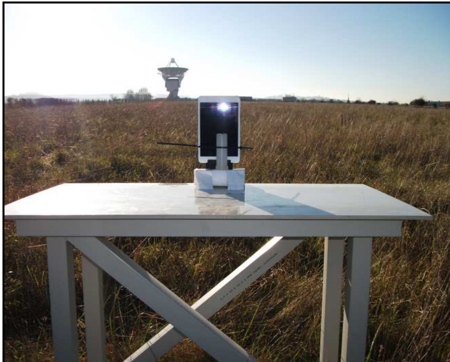
Set up for 300 metre measurements (EUT end facing towards the mag loop antenna)
