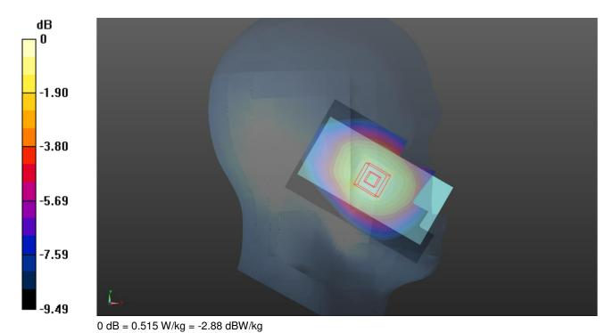
Communication System: UID 0, GSM 850 MHz; Frequency: 836.6 MHz; Duty Cycle: 1:8.3
