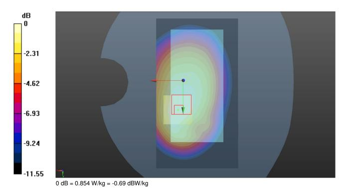
Communication System: UID 0, GPRS 850 MHz 2TX; Frequency: 848.8 MHz; Duty Cycle: 1:4
