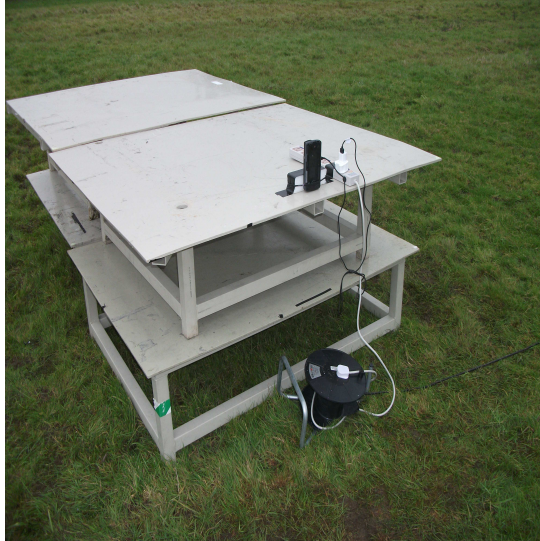
Set up for 300 metre measurements (EUT end facing away from the mag loop antenna)
