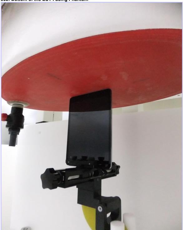
003: Bottom of the EUT Facing Phantom with Infinea Tab Case
