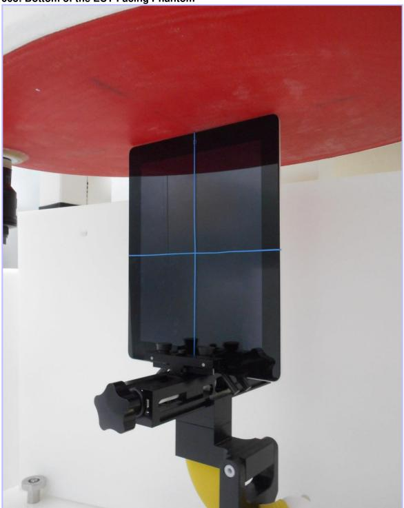
004: Back of the EUT Facing Phantom with Infinea Tab Case
