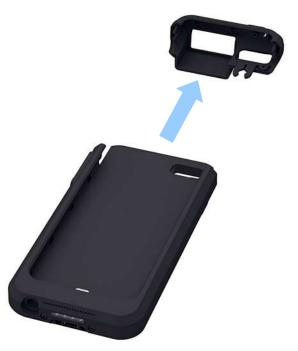
**Step 2** – Slide the iPod 5 or iPhone 5 into Linea Pro 5. (Please, before attaching the device, check the compatibility version of the Linea Pro 5 - for iPod 5 or iPhone 5 (page 10), and then connect it with the correct Linea Pro 5).
