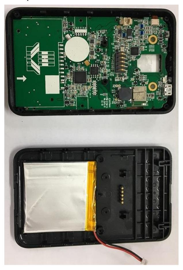
2. With removed top cover. Contactless Reader antenna position.
