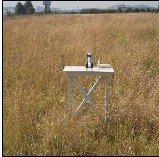
Set up for 300 metre measurements (EUT end facing towards the mag loop antenna)
