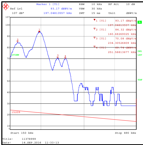
150 kHz to 490 kHz / average detector / EUT operating / measured at 30 metres on an open field test site
