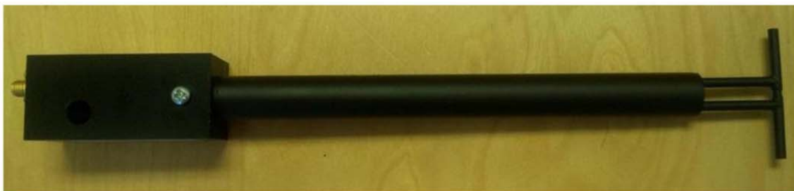
Figure 1 – MVG COMOSAR Validation Dipole
