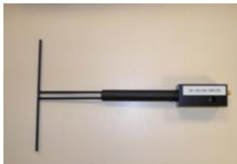
Figure 1 – Satimo COMOSAR Validation Dipole
