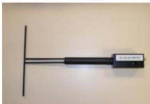
Figure 1 – Satimo COMOSAR Validation Dipole
