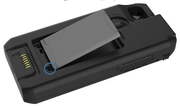
Direction of battery cover closing. Place the clips to correct position.
