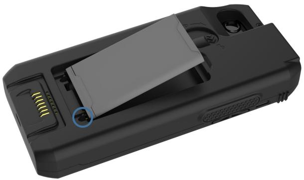
Insert first the side with contacting pads of the battery then press it down.
