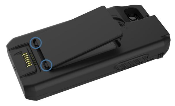
When the battery cover is completely closed, slide the lever to lock position.
