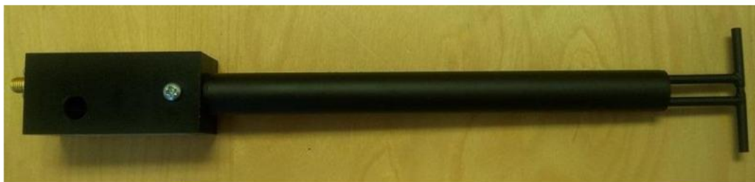
Figure 1 – MVG COMOSAR Validation Dipole
