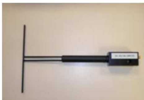
Figure 1 – Satimo COMOSAR Validation Dipole
