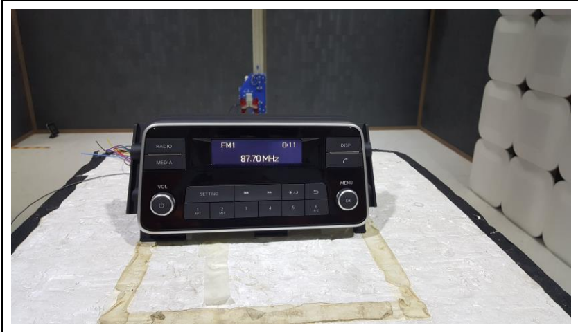
EUT Position: Y-axis
