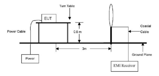
The diagram below shows the test setup that is utilized to make the measurements for emission from 30 Mz to 1 Gz emissions.
