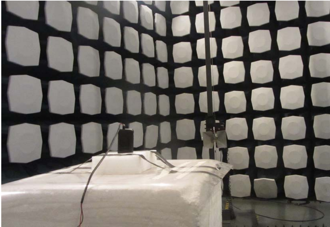
Picture 2: Radiated Spurious Emissions Test setup
