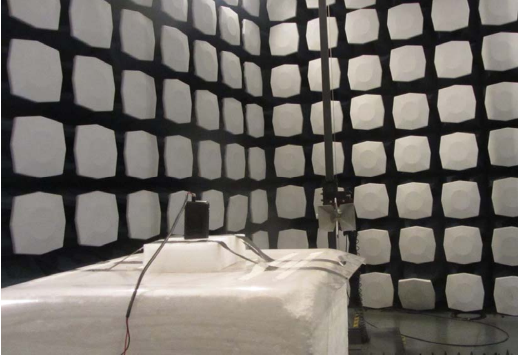
Picture 2: Radiated Spurious Emissions Test setup
