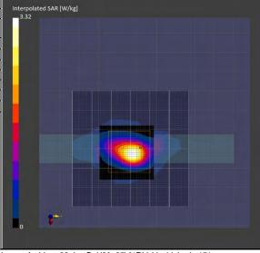
\*. Date tested: 2024-01-12;Tested by: Hiroshi Naka; Tested place:No.7 shielded room; Ambient: 22 deg.C. / (60–65) %RH; Liquid depth: 151 mm; \*. Liquid temperature: 22.0 deg.C. ± 0.5 deg.C. (22.5 deg.C., in check); \*. Red cubic: big=SAR(10g) / small=SAR(1g) \*. Project file name-Measurement Group: 240110\_14926563\_h248.5g\_p53.d8sar-1/12-2,5h28,at1,side,n20(m0),5825 Remarks:
