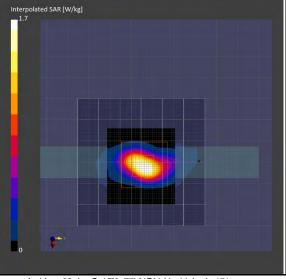
\*. Date tested: 2024-01-12;Tested by: Hiroshi Naka; Tested place:No.7 shielded room; Ambient: 23 deg.C. / (70–75) %RH; Liquid depth: 151 mm;
