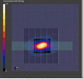
\*. Date tested: 2024-01-11;Tested by: Hiroshi Naka; Tested place:No.7 shielded room; Ambient: 23 deg.C. / (65~75) %RH; Liquid depth: 151 mm;
