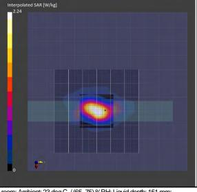
\*. Date tested: 2024-01-11;Tested by: Hiroshi Naka; Tested place:No.7 shielded room; Ambient: 23 deg.C. / (65~75) %RH; Liquid depth: 151 mm; \*. Liquid temperature: 22.0 deg.C. ± 0.5 deg.C. (22.5 deg.C., in check); \*. Red cubic: big=SAR(10g) / small=SAR(1g) \*. Project file name-Measurement Group: 240110\_14926563\_h248.5g\_p53.d8sar-1/11-24,5h17,at1,side,a,5500 Remarks:
