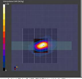
\*. Date tested: 2024-01-11;Tested by: Hiroshi Naka; Tested place:No.7 shielded room; Ambient: 23 deg.C. / (65~70) %RH; Liquid depth: 151 mm;
