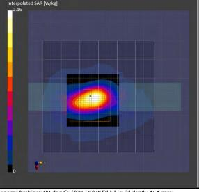
\*. Date tested: 2024-01-16;Tested by: Hiroshi Naka; Tested place:No.7 shielded room; Ambient: 23 deg.C. / (60~70) %RH; Liquid depth: 151 mm;
