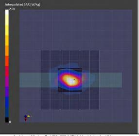
\*. Date tested: 2024-01-11;Tested by: Hiroshi Naka; Tested place:No.7 shielded room; Ambient: 23 deg.C. / (70–75) %RH; Liquid depth: 151 mm; \*. Liquid temperature: 22.0 deg.C. ± 0.5 deg.C. (22.5 deg.C., in check); \*. Red cubic: big=SAR(10g) / small=SAR(1g) \*. Project file name-Measurement Group: 240110\_14926563\_h248.5g\_p53.d8sar-1/11-21,5h14,at1,side,a,5180 Remarks:
