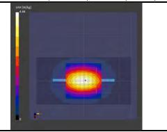
\*. Date tested:2024-01-12; Tested by: Hiroshi Naka; Tested place:No.7 shielded room; Ambient: 23 deg.C. / (65~75) %RH; Liquid depth: 151 mm; \*. Liquid temperature: 22.0 deg.C. ± 0.5 deg.C. (22.5 deg.C., in check); \*. Red cubic: big=SAR(10g) / small=SAR(1g) \*. Project file name-Measurement Group: 240110\_14926563\_h24&5g\_p53.d8sar-1/12a,50mw Remarks:
