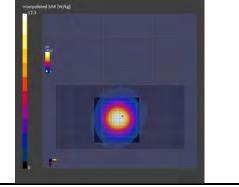
\*. Date tested:2024-01-12; Tested by: Hiroshi Naka; Tested place:No.7 shielded room; Ambient: 23 deg.C. / (65~75) %RH; Liquid depth: 151 mm; \*. Liquid temperature: 22.0 deg.C. ± 0.5 deg.C. (22.5 deg.C., in check); \*. Red cubic: big=SAR(10g) / small=SAR(1g) \*. Project file name-Measurement Group: 240110\_14926563\_h24&5g\_p53.d8sar-1/12d,50mw Remarks:
