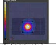
\*. Date tested:2024-01-12; Tested by: Hiroshi Naka; Tested place:No.7 shielded room; Ambient: 23 deg.C. / (65~75) %RH; Liquid depth: 151 mm; \*. Liquid temperature: 22.0 deg.C. ± 0.5 deg.C. (22.5 deg.C., in check); \*. Red cubic: big=SAR(10g) / small=SAR(1g) \*. Project file name-Measurement Group: 240110\_14926563\_h24&5g\_p53.d8sar-1/12c,50mw Remarks:
