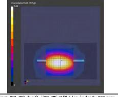
\*. Date tested:2024-01-15; Tested by: Hiroshi Naka; Tested place:No.7 shielded room; Ambient: (22-23) deg.C. / (60-75) %RH; Liquid depth: 151 mm;
