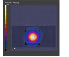
\*. Date tested:2024-01-15; Tested by: Hiroshi Naka; Tested place:No.7 shielded room; Ambient: (22-23) deg.C. / (60-75) %RH; Liquid depth: 151 mm; Remarks:
