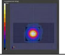
\*. Date tested:2024-01-12; Tested by: Hiroshi Naka; Tested place:No.7 shielded room; Ambient: 23 deg.C. / (65~75) %RH; Liquid depth: 151 mm; \*. Liquid temperature: 22.0 deg.C. ± 0.5 deg.C. (22.5 deg.C., in check); \*. Red cubic: big=SAR(10g) / small=SAR(1g) \*. Project file name-Measurement Group: 240110\_14926563\_h24&5g\_p53.d8sar-1/12b,50mw Remarks:
