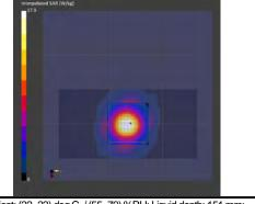
\*. Date tested:2024-01-11; Tested by: Hiroshi Naka; Tested place:No.7 shielded room; Ambient: (22-23) deg.C. / (55-70) %RH; Liquid depth: 151 mm; \*. Liquid temperature: 22.0 deg.C. ± 0.5 deg.C. (22.5 deg.C., in check); \*. Red cubic: big=SAR(10g) / small=SAR(1g) \*. Project file name-Measurement Group: 240110\_14926563\_h24&5g\_p53.d8sar-1/11d,50mw Remarks:
