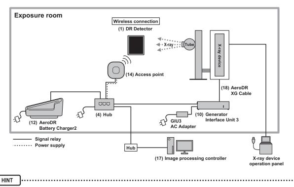
• The Generator Interface Unit 3 can also be powered from the GIU3 AC Adapter.
