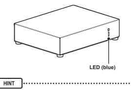
• When using the GIU3 AC Adapter, confirm that the Generator Interface Unit 3 is turned on when the power plug is connected to a wall outlet and the LED (blue) lights.
