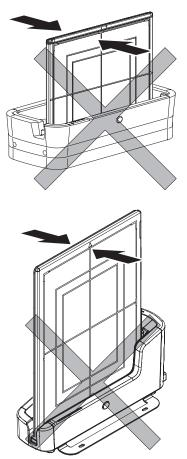
— The DR Detector is precision equipment, and therefore impact or vibration during radiography or image transfer may affect the image quality. Be careful when handling the DR Detector during and just after radiography.
