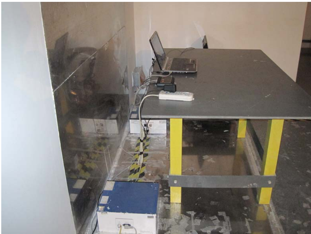
Conducted Emissions Test Setup Side View
