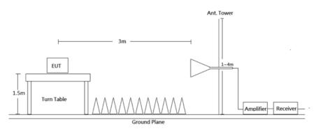
Radiated emission tests were performed in the 3 meters chamber test site, using the setup accordance with the ANSI C63.10-2013. The specification used was the FCC Part 15.209 and FCC 15.247 Limits.
